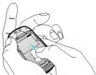
To insert the SIM card
