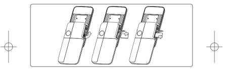
**Remove the memory card**: Open the rubber cap and gently push the memory card until unlocked. Take out your MicroSD card and close the cap.
