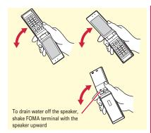
③ Swing FOMA terminal in about 10 times against dry, clean cloth etc. to wipe off water remaining in the microphone, earpiece, speaker, keypad, hinges or charging jack, etc.
