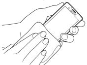
Securely hold the terminal and shake it approx. 20 times until there is no more water splattering
