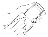
Securely hold the FOMA terminal and shake it approx. 20 times until there is no more water splattering
