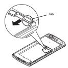
3 Place the UIM on the tray, setting the IC surface on the downside.
