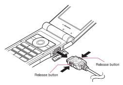
Remove the FOMA USB Cable with Charge Function 02 from the USB terminal of the PC
