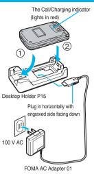
Charge with the AC adapter only Insert the connector with the engraved surface facing up until it clicks. Pull straight the connector out while pressing the release buttons.
