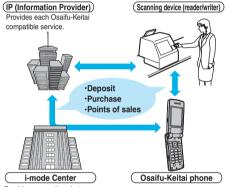
Provides connections between the information provider and i-mode phones.
