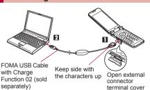
Insert the FOMA side of the FOMA **USB Cable with Charge Function 02** (sold separately) into the external connector terminal on the FOMA terminal ( 11).
