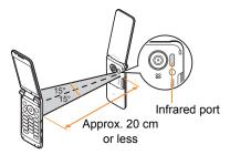
Face the infrared ports of the receiver's and sender's FOMA terminal each other and set the distance between them to approximately 20 cm or less.
