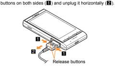
Do not forcibly insert or remove. May cause damage to the external connector terminal and the connector or result in malfunction.
