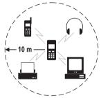
Every Bluetooth™ device has a unique address and a name. This guarantees a connection between the intended communication partners. The security concept is based on a password that both devices exchange when they connect for the first time. These "trustworthy" partners can be included in a list. The password prompt is not required for future connections. For settings, see page 95.
