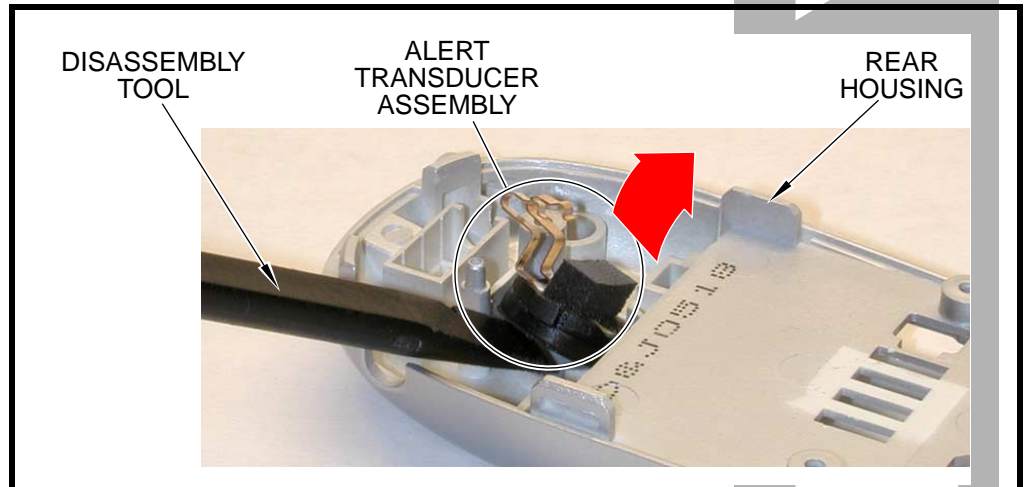
Figure 13. Removing the alert transducer assembly
