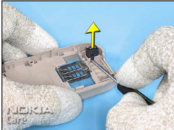
14. Lift the MICROPHONE from its position and remove it.
