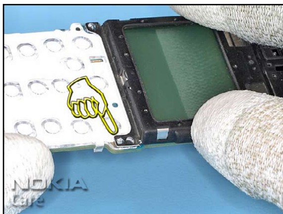
3. Align the UI SHIELD with the guide pin of the KEYMAT LIGHTGUIDE ASSY.
