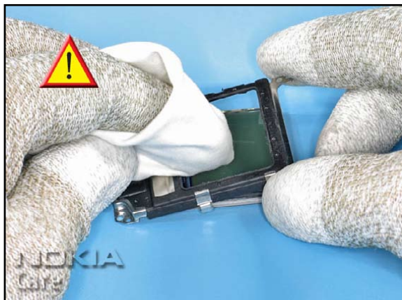
10. Carefully push out the LCD from the UI SHIELD using a clean cloth. Cover the LCD with the protective film.
