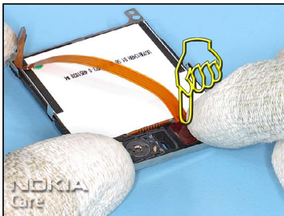
2. Gently connect the FPC LINK to the LCD connector.
