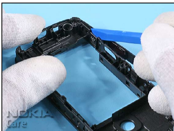
33. Separate the other side of the DECO TRIM from the B-COVER...
