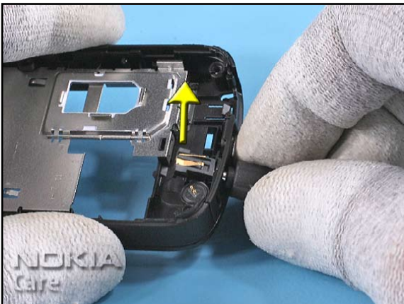
23. Use the DC plug to remove the DC-JACK.
