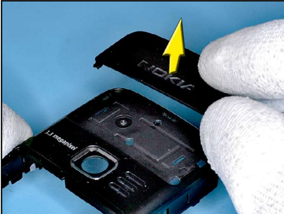
37. Remove the TOP COVER from the B-COVER.
