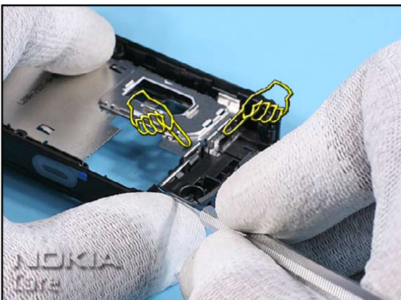
29. Finally, release the both clips on the lower side of the B-COVER and remove the LABEL COVER ASSY.
