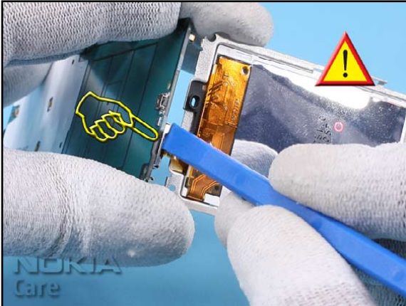
13. Turn the UI-SHIELD ASSY to the position shown and carefully open the LCD connector.
