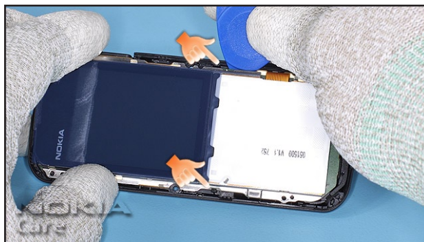
10. The C-COVER and PWB are secured by two clips to the D-COVER. Unlock the clips and remove the parts from the D-COVER.
