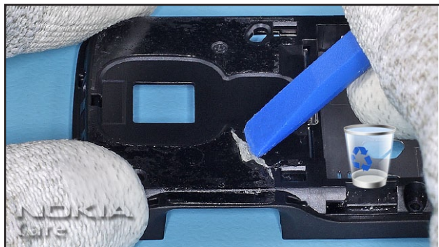
22. Remove the ADHESIVE residues and discard it.
