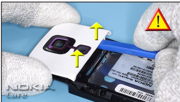
21. Use the SS-93 as a lever to remove the B-DECO COVER.
