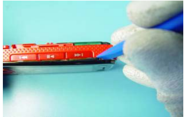
8) Pry open the clips of the A-COVER ASSY.
