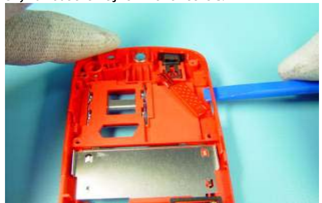
34) Push out the MEMORY CARD DOOR with the SS-93.
