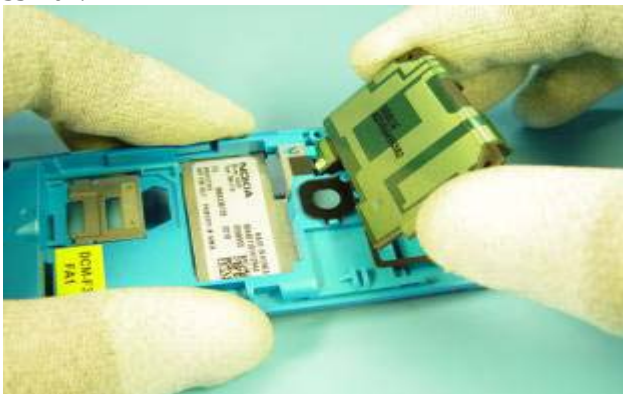
27) Unlock and remove the CAMERA MODULE with the SS-102.
