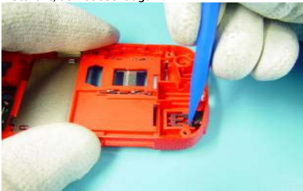
33) Ease out the MICROPHONE with the dental pick. Discard it, do not use it again.
