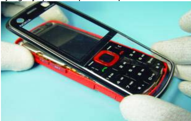
9) Slightly open the clips at the top...
