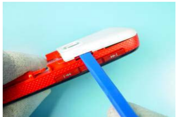
4) Gently release the clip of the ANTENNA COVER ASSY, beginning at the shown side.
