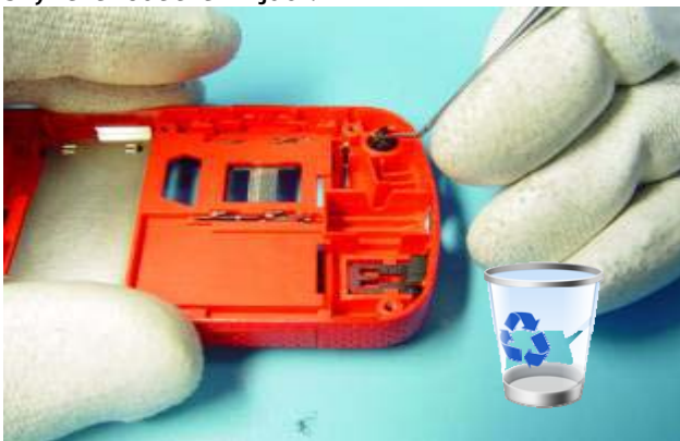
33) Ease out the MICROPHONE with the dental pick. Discard it, do not use it again.
