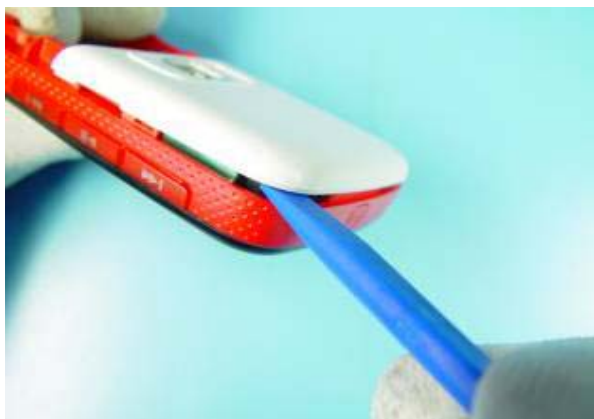
5) Also release the clips at the top...
