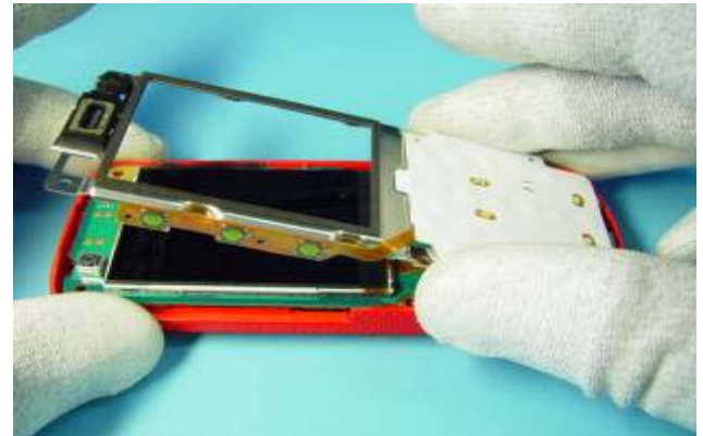
16) Lift up the DISPLAY FRAME ASSY. Note that the flex foil is still connected.
