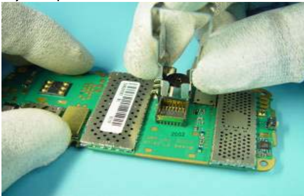
27) Unlock and remove the CAMERA MODULE with the SS-102.
