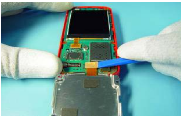
17) Carefully open the flex connector.
