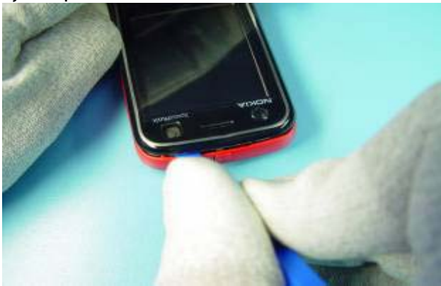
9) Slightly open the clips at the top...
