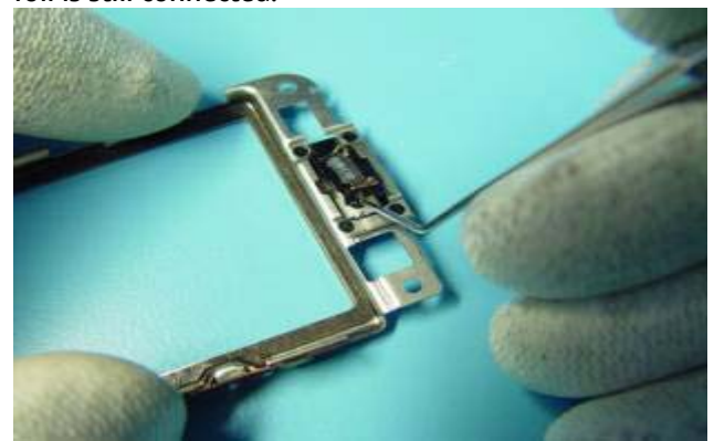
16) Lift up the DISPLAY FRAME ASSY. Note that the flex foil is still connected.
