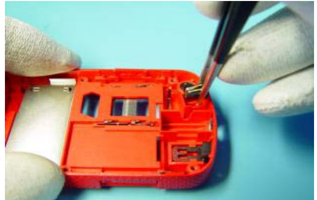
32) Pull out the DC JACK with tweezers.
