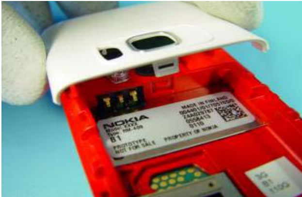
7) Lift up the ANTENNA COVER.
