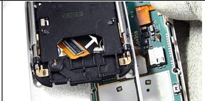
34.) Separate the Slide Assembly from the B-Cover Assembly slowly not to damage the Main Flex.
