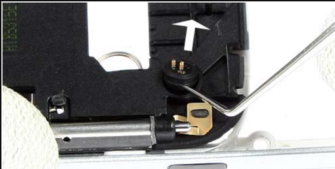
35.) Remove the Microphone with the Dental Tool.
