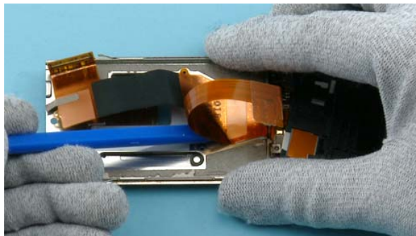
45) Continue to release the remaining part of the MAIN FLEX ASSEMBLY on the top side.
