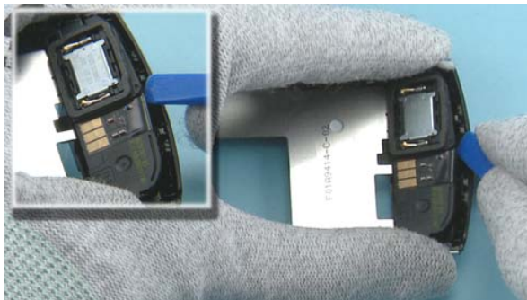
17) Use the SS-93 to release the ANTENNA MODULE ASSY.
