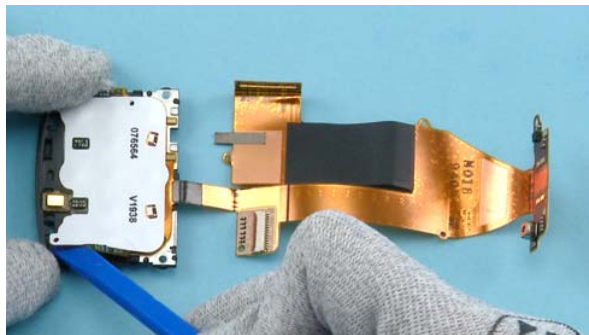
47) Remove the main flex from the UI KEYMAT SUPPORT ASSEMBLY with the SS-93.
