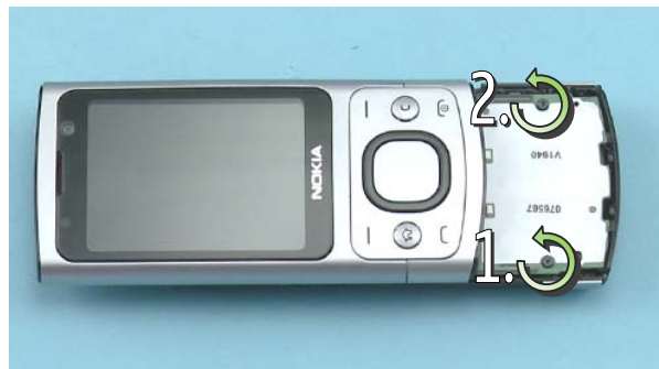
10) Slide the phone open. Unscrew the two TORX+ size 4 screws in the order shown.
