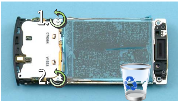
35) Unscrew the two TORX+ size 4 screws in the order shown. Do not use them again. Discard them.
