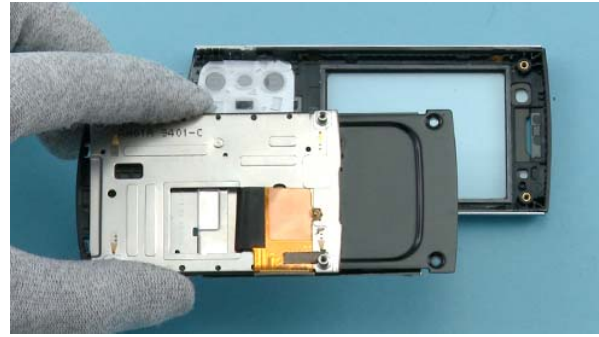
32) Lift up the SLIDE MODULE ASSY, and remove the A-COVER.
