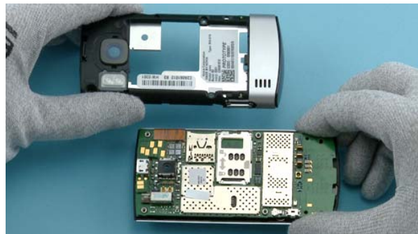
12) Close the slide. Lift up and separate the D-COVER ASSY.
