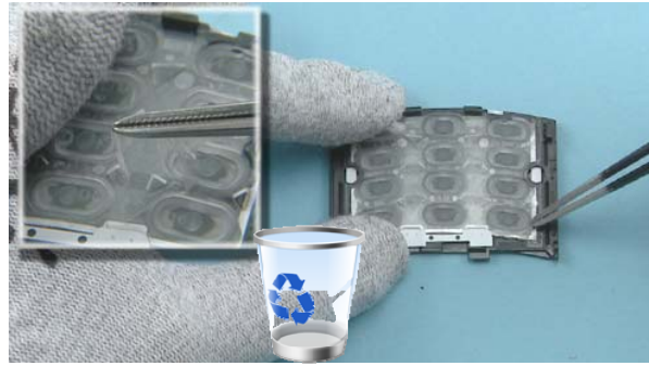
8) Use the tweezers to remove the MAIN KEYMAT ADHESIVE. Do not use it again. Discard it.
