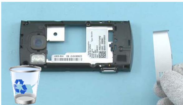
21) Remove the ANTENNA COVER. Do not use it again. Discard it.
