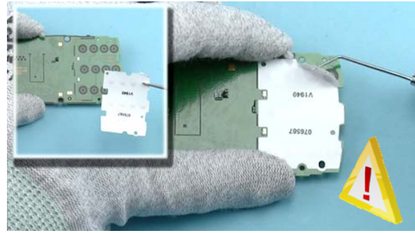
26) Use the dental tool to lift up one corner of the DOMESHEET. Peel off and remove the DOMESHEET ASSY with fingers. Do not use it again. Discard it. Be aware of the sharp point of the dental tool – be careful not to injure yourself!
