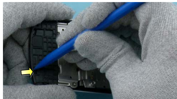
30) Then release the clips at the bottom end.
