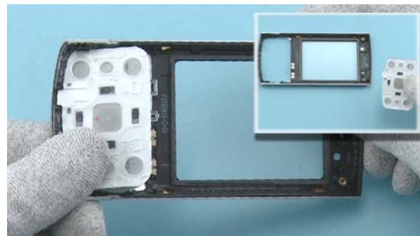
34) Press out and remove the UI KEYMAT ASSEMBLY.
