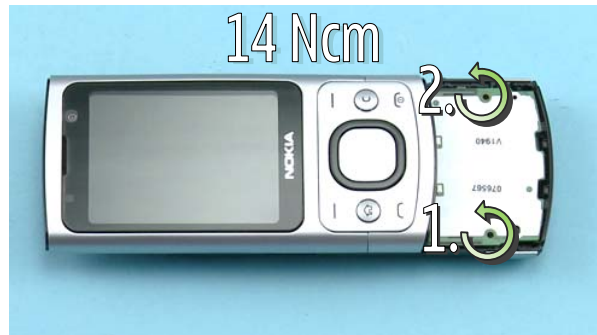
4) Tighten the two TORX+ size 4 screws to the torque of 14 Ncm in the order shown.
