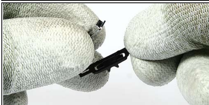
27. Separate the VOLUME KEY ACTUATOR from the VOLUME KEY.
