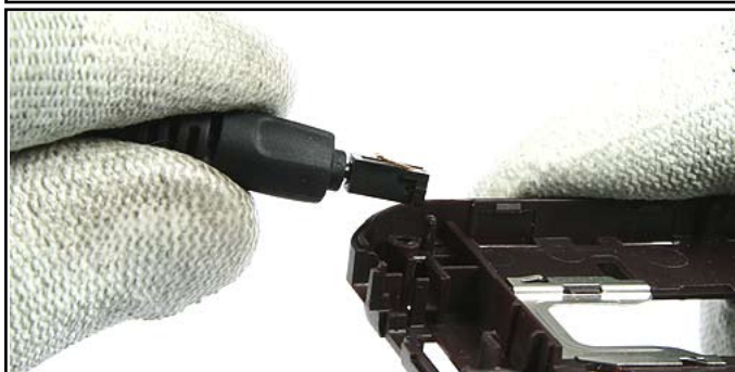
31. Remove the DC-JACK with a DC PLUG.
