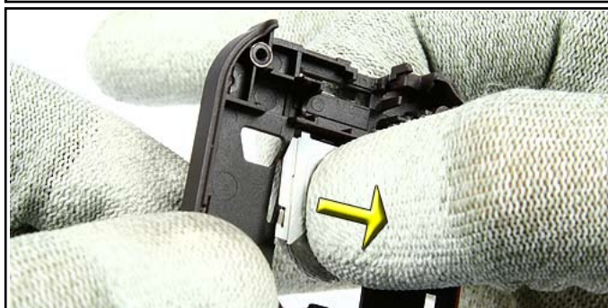
32. Press the SIM-GRIP in the shown direction, and lift one side of it out of the B-COVER ASSY.
