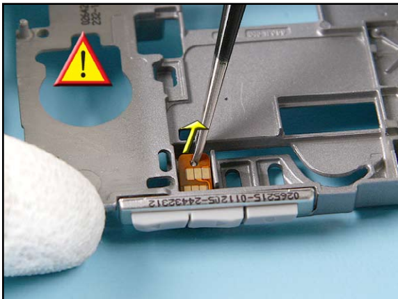
25. Unlock the SIDE BUTTON MODULE ASSY...
