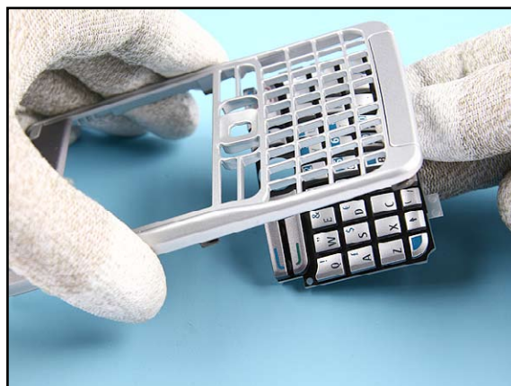
16. Separate the KEYMAT from the A-COVER ASSY.
