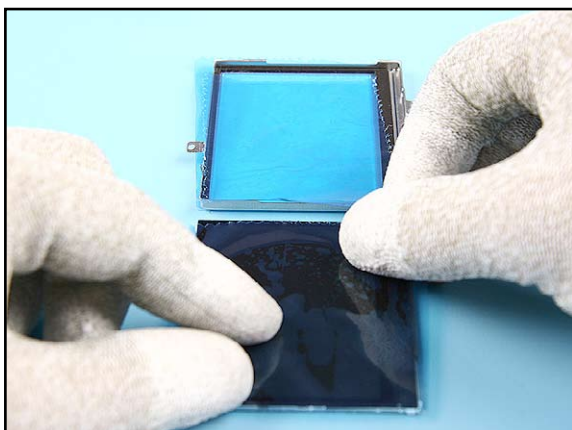
15. Remember to cover the inner side of the WINDOW ASSY and the LCD MODULE with protective film.
