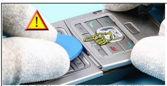
41. Place the SRT-6 between the C-COVER and the D-COVER as shown and lift the C-COVER a bit. Do not slide the SRT-6 along the
