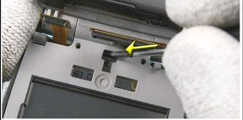
24. Then, release the snap in the middle of the cover with a slotted screwdriver.
