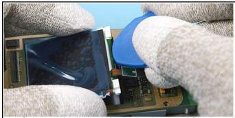
17. Lift the LCD a bit by using the SRT-6 and remove it from its mounting.
