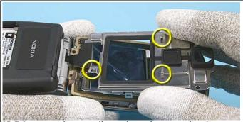
15. Take care to the grounding springs when removing the SHIELD LID ASSY.
