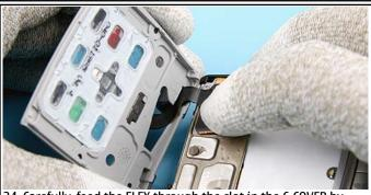
24. Carefully, feed the FLEX through the slot in the C-COVER by securing the closed connector.
