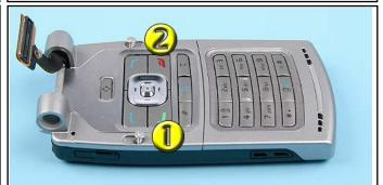
28. To prevent damaging the plastic threads, turn the SCREWS slightly left first. Then tighten them in the shown order with a torque setting of 17Ncm.
