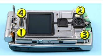
47. To prevent damaging the plastic threads, turn the screws slightly left first. Then tighten them in the shown order with a torque setting of 17Ncm.
