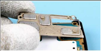
45. Remove the SHIELD KEY.
