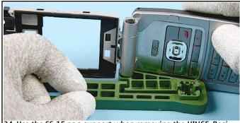
34. Use the SS-15 as a support when removing the HINGE. Position the HINGE exactly over the recess.
