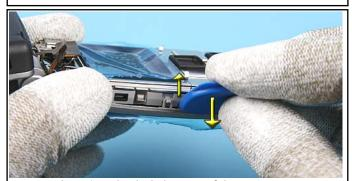
13. Open the unit and unlock the snap of the B-COVER ASSY.
