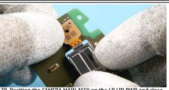
38. Position the CAMERA MAIN ASSY on the LR LID PWB and close the CAMERA connector.
