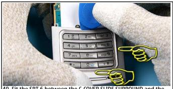
49. Fit the SRT-6 between the C-COVER SLIDE SURROUND and the C-COVER and unlock the C-COVER SLIDE SURROUND.
