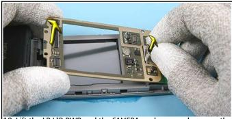
18. Lift the LR LID PWB and the CAMERA as shown and remove the modules carefully.
