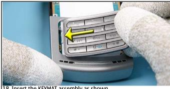
18. Insert the KEYMAT assembly as shown.
