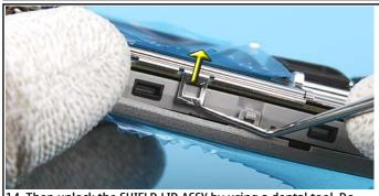
14. Then unlock the SHIELD LID ASSY by using a dental tool. Do the same on both sides.
