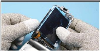
29. Protect the LCD with a film and remove it from the LID CENTER FRAME.
