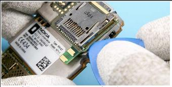
61. Carefully, disconnect LZ BT MODULE from the ENGINE BOARD.
