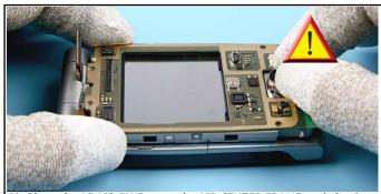
41. Place the LR LID PWB onto the LID CENTER FRAME and check the position of the CAMERA MAIN ASSY.
