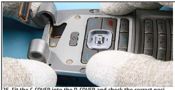
25. Fit the C-COVER into the D-COVER and check the correct position of the FLEX.
