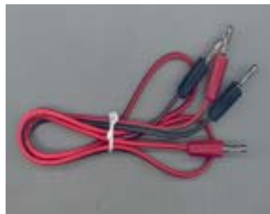
3-3-4. Power Supply Cable
