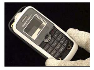
Insert the guitar pick at the bottom of the phone and slide it towards the top to release the three snap hooks.
