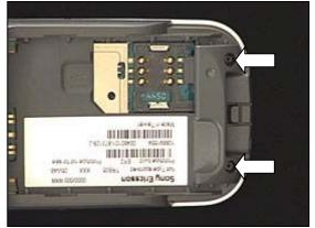
Press simultaneously on these four spots. Check on both sides that the *front cover* is snapped to the rear cover.
