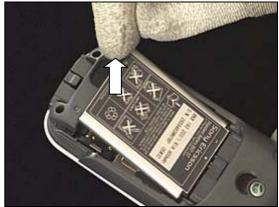
and slide the *battery cover* until it becomes released and can be removed.
