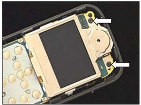
Press simultaneously on both sides of the *PBA* where the snap hooks of the rear cover are located.
