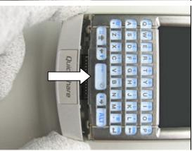
Apply **15 Ncm**  $\pm$  2 Ncm of torque for the two <u>new</u> screws by using the JCIS bit!
