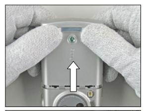
Slide down the *battery lid* from its mounted position towards the bottom of the phone and remove it.
