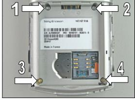
Apply **24 Ncm**  $\pm$  2 Ncm torque when tightening the two screws using torx bit no. 6! (can be reused if not damaged)
