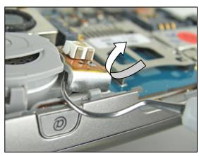
Use the front opening tool to bend under the *antenna/acoustic* until it becomes loose.
