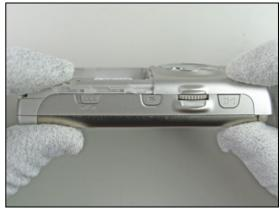
Apply **15 Ncm**  $\pm$  2 Ncm torque when tightening two <u>new</u> screws (1 and 2) using torx bit no. 6!
