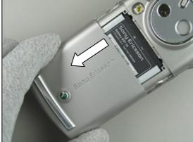
Start to remove the *battery* from the phone with your fingers or the front opening tool.
