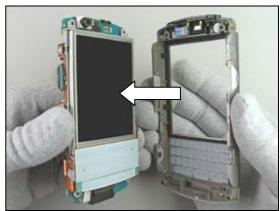
Place the top of the PBA/LCD into the top of the *cabinet upper sub*.
