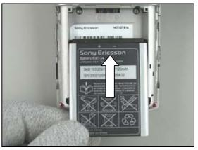
Slide the *battery* all the way inside the battery compartment and press it down at the bottom.
