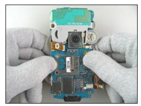
Make sure that the *main PBA* is in the right position, and properly latched by the four hooks (two on each side of the frame).
