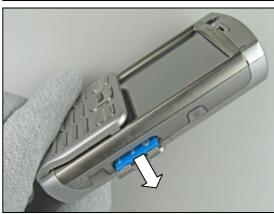
How to open a board-to-board connector with the front opening tool.
