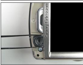
Correctly mounted camera bezel.
