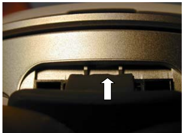
The location of the first Liquid Intrusion Indicator. (Remove or fold-back system connector cover)
