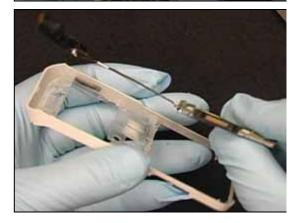
Remove the antenna from the slot on the rear frame.
