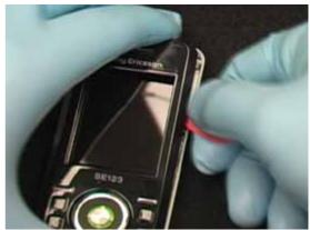
Slide the plectrum toward the top corner to release the latch.
