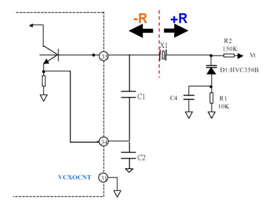
HD155155NP provides a VCXO function. With that function, we can build a reference clock generation circuits as shown in the above graph. This means that the VCTCXO module is not necessary for clock application, and only one crystal with 8ppm tolerance and one variocap are enough.
