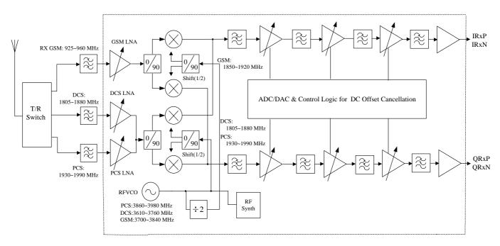
The Receiver structure in HD155155NP is a zero-IF solution. That means RF signal is directly down-converted to the baseband signal. And by the way, all of the DC-offset canceling processes are done within chip. We do not have to care about that.
