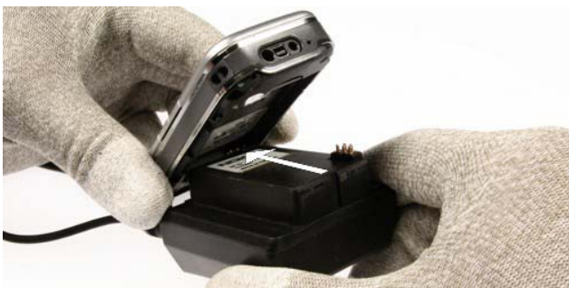
Insert the Flash Adapter SF-10 like a battery, start at the Battery Connector side.
