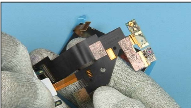
43. Keep these adhesives clean if this part should be reused. Also remove the adhesive residues on the opponent part.
