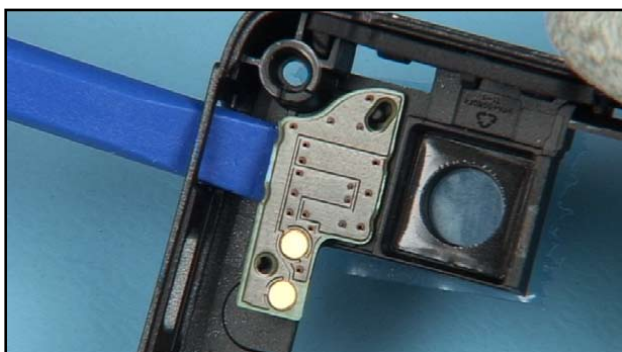
53. Lever out the FLASH ASSEMBLY. Keep the adhesive clean if this part should be used again.
