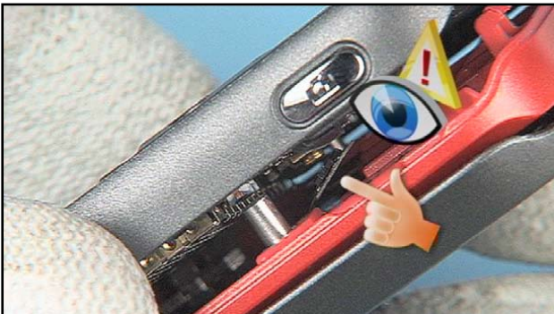
13. Note that this small flex connector was opened before continuing.
