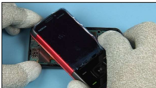
44. Gently lift up and flip the upper part over the D-COVER.
