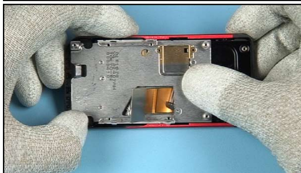
32. Shift open the SLIDE MODULE ASSEMBLY.
