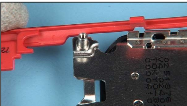
23. Shift the LOWER BEZEL ASSEMBLY into direction of the threads. It can be lifted up now.
