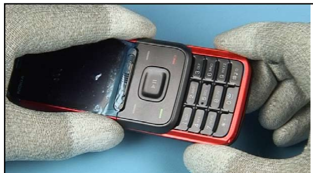
60. Check the correct placement of the keymat.
