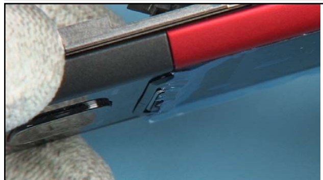
24. Prevent mechanical stress to the NAVI SLIDER MODULE while unscrewing the screws.
