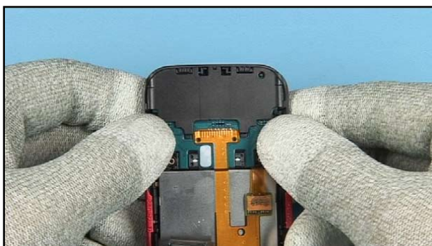
29. Carefully bend the A-COVER on both sides...
