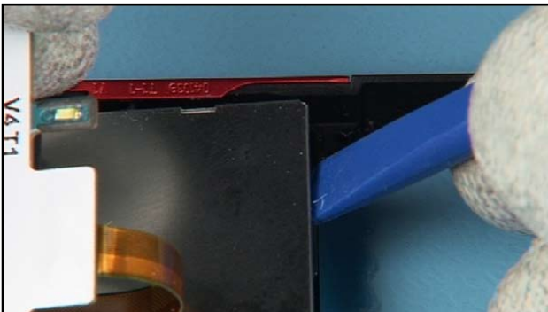
35. Release the LCD from its sealing with the SS-93 partly.
