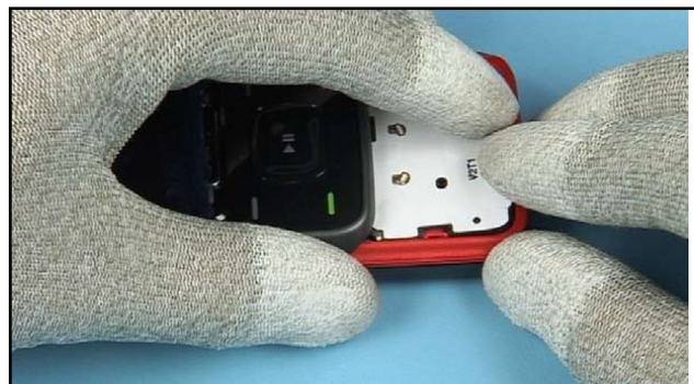
52. Smooth down the BOTTOM KEYMAT SUPPORT evenly. Click the clips into their places.
