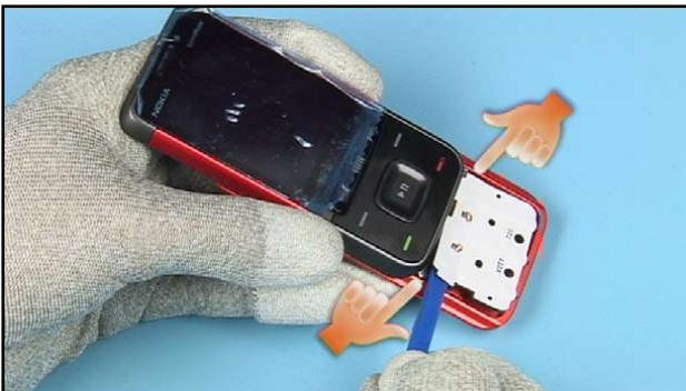
19. The BOTTOM DOMESHEET was glued in at the SLIDE MODULE ASSEMBLY. Gently release the domesheet on both sides.
