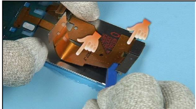
42. Release the adhesive pads of the TOP FLEX ASSEMBLY, beginning at this edge. Also release the other shown pads.
