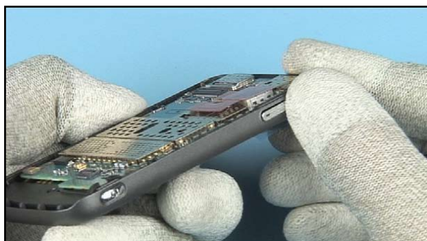
12. Check that all keys operate before going on.
