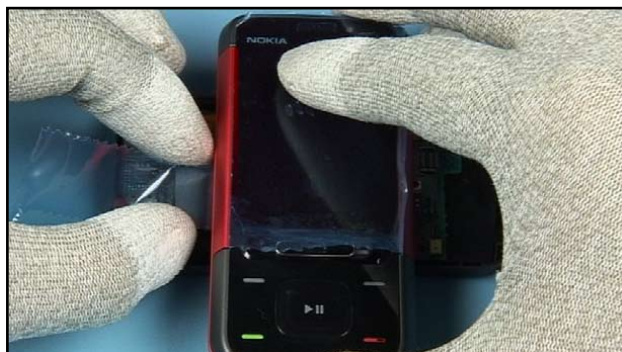
42. Hold the flex connector. Bring the upper part into position over the lower part as shown.
