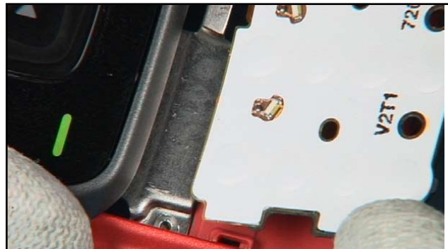
20. Now the BOTTOM DOMESHEET can be removed. Remove any adhesive residues from the opponent part.
