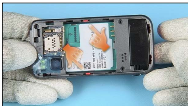
46. Check the correct positioning of both clips before going on.
