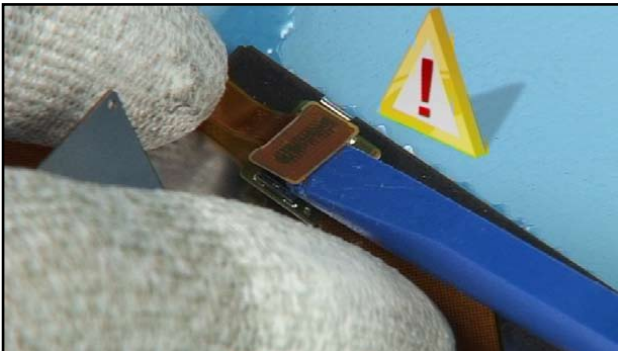
41. Do not apply pressure at the components underneath. Gently lever up the flex connector.
