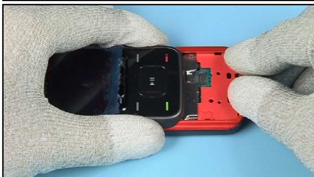
47. Shift open the assembly. Click these bottom clips into their places. Check the correct alignment of the cover parts.
