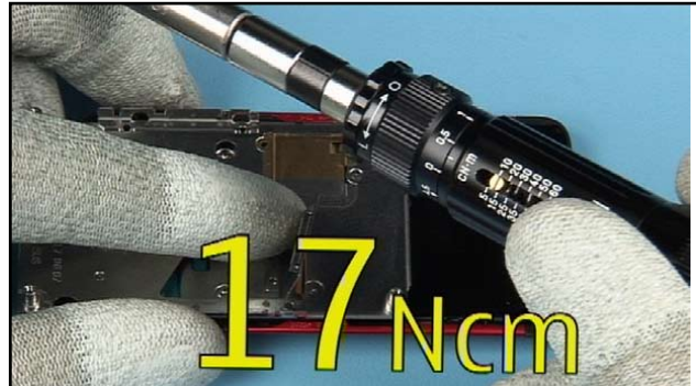
34. Set the correct torque.
