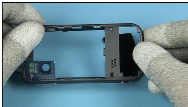
50. Turn the D-COVER. Simply let drop out the ANTENNA IHF ASSEMBLY.
