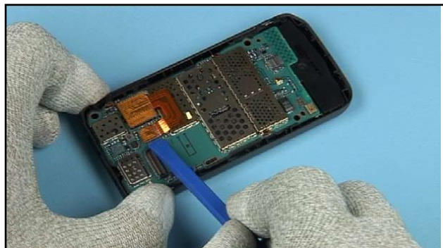
44. Continue with the lower assembly. Use the SS-93 for opening the flex connector of the CAMERA FLEX MODULE.
