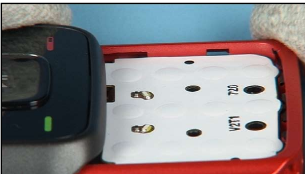
53. Check the correct positioning of the BOTTOM KEYMAT SUPPORT before going on.
