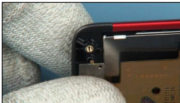
18. Slightly push the CMOS CAMERA and this guide pin into its place.
