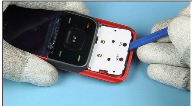
18. Turn the assembly. Gently lift up the BOTTOM KEYMAT SUPPORT.
