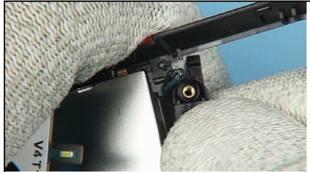
34. ...until this large clip was released partly. Now pull it out sideways to release the clip completely.
