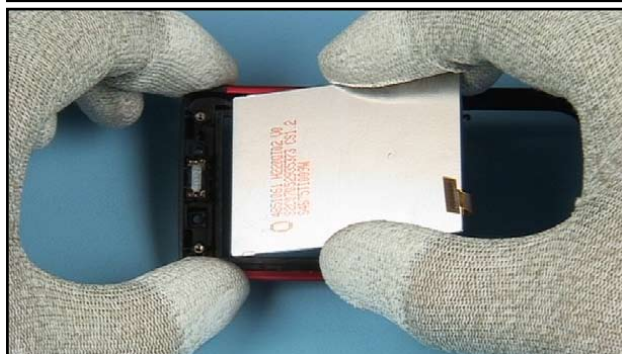
16. Align the LCD to the top guide. Smooth it down evenly.
