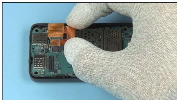
10. Check the camera window for cleanliness. Insert the CAMERA FLEX MODULE into its compartment.
