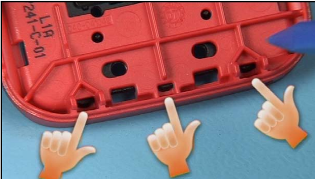
17. Unlock these 3 plastic clips with the SS-93.
