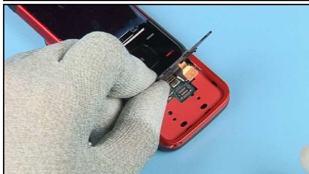
48. Bring the BOTTOM KEYMAT SUPPORT into position as shown.
