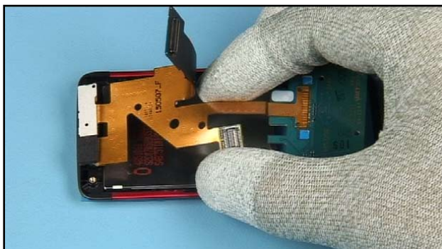
17. Place the TOP FLEX ASSEMBLY. Remove the protective film before if this part is new.
