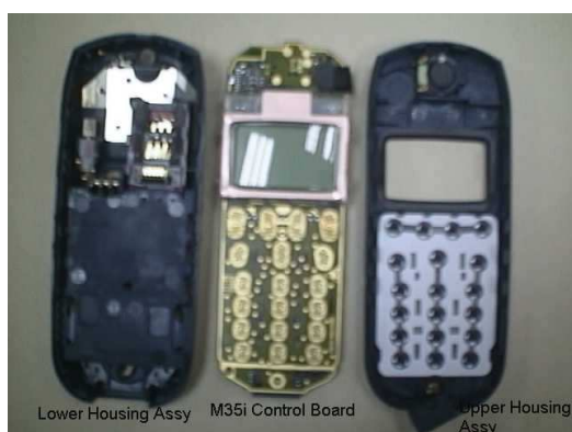
PHOTO 2.23 ASSEMBLE M35i – STEP 1
