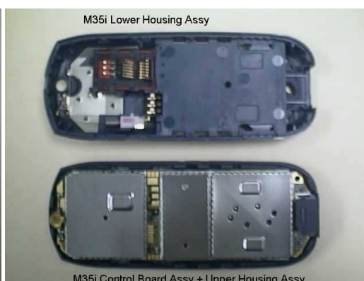
PHOTO 2.24 ASSEMBLE M35i – STEP 2
