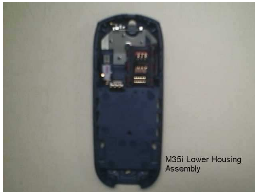
PHOTO 2.12 Lower Housing Assy – STEP 1
