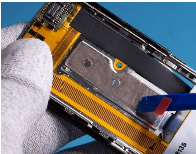
3) Remove the section foil by lifting the red tab to expose the glued area.
