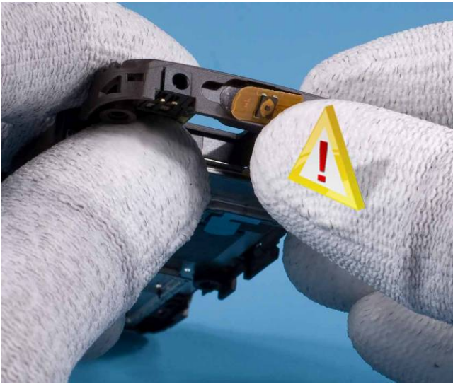
5) Carefully bend the power key area into place and press home.
