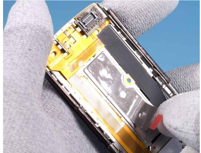
2) Replace this section with Display Panel Adhesive Light CC . This is necessary to ensure a correct display fixation to the Slider Module and a correct grounding of the display.
