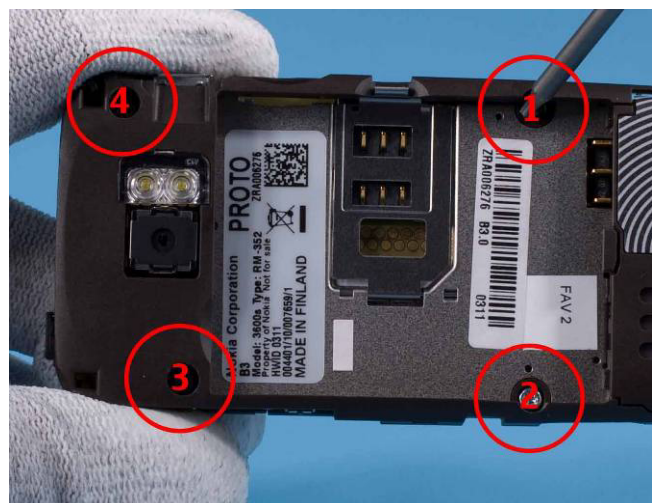
18) Unscrew the 4 remaining screws.
