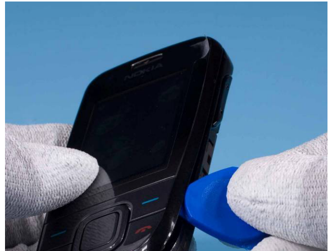
4) Open the first cover clip from the A-Cover with SRT-6.
