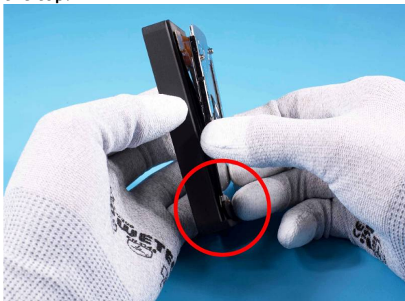
3) Align the bottom edge of the slider to the bottom edge of the JIG as shown and press down firmly.
