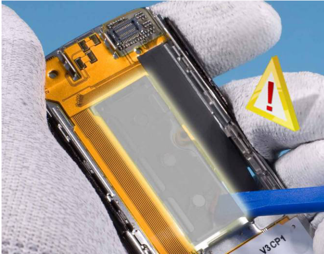
1) Remove the LCD as shown in disassembly instruction. Remove the shaded area from UI Flex Assy . Take care not to damage the UI Flex Assy itself.
