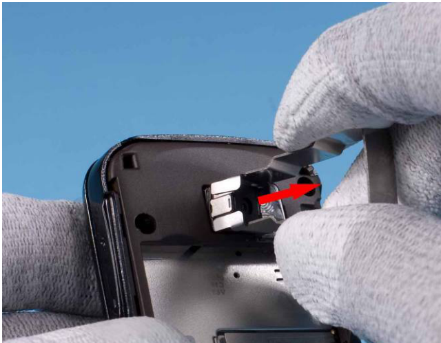
3) Remove the Camera Module with SS-102.
