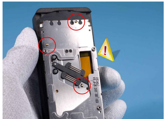
4) Make sure the guide pins are aligned correctly.
