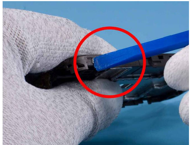
2) If the D-Cover is re-used: Remove any glue residue. There are three areas to clean: the Side Keys/AV Connector/Power Switch.
