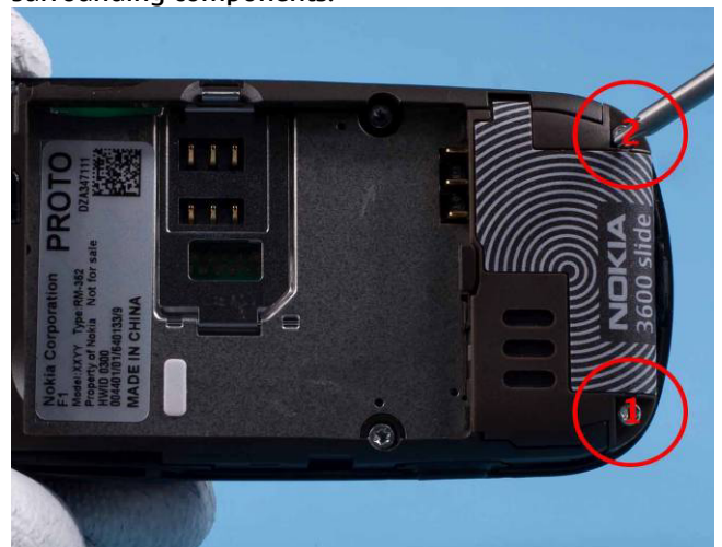
12) Unscrew the 2 screws from the Antenna Cover Assy .
