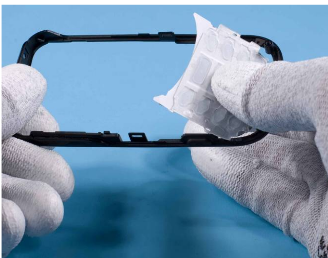
17) Separate the Numeric Keymat from the E-Cover.
