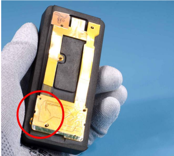
1) Place the UI Flex Assy onto the JIG. Note that the B2B Connector is under the assy and not on the top.
